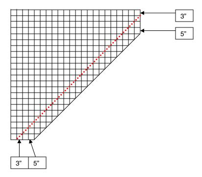
9. Mark the positions for the pins along the newly drawn line. Mark the halfway point of each division. Mark the  $\frac{1}{4}$  mark for each division as well. Insert a pin at each of the marks.
