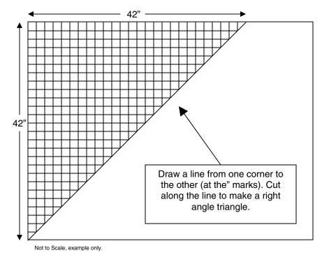
3. Draw a line from one corner to the other (at the 42" marks). Cut along the line to make a right angle triangle.
